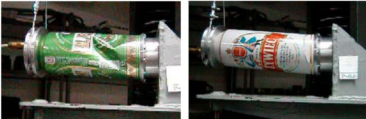
Fig. 4 Deformation of the beverage can loaded by pressure: a) 0 MPa, b) 0,35 MPa
